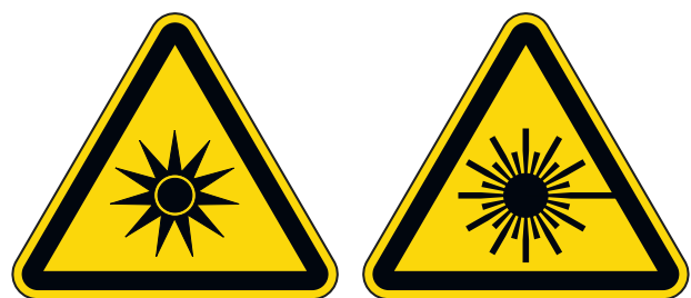
FIG. 2 Warning sign against optical radiation (left) and warning sign against laser radiation (right) (Graphic: C. Prall, smart optics Sensortechnik GmbH).
