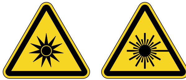
Figure 2: Warning sign against optical radiation (left) and warning sign against laser radiation (right) Graphic: C. Prall, smart optics Sensortechnik GmbH
